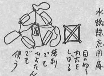
Mizugumo application. Tie up logs as shown. Sake containers or gourds could also be used.
